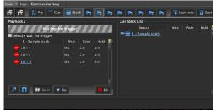
We are putting the cue stack number one into playback two. This will not lead into any action yet since no cue is triggered. The command for this is
